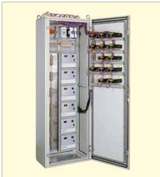
Internal view of the CMR Panel. An isolator, fuses, power supply, computer interface terminals and six DPC200 Controllers are fitted on the back plate. All factory tested.
