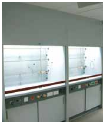
Typical Fume Cupboard
